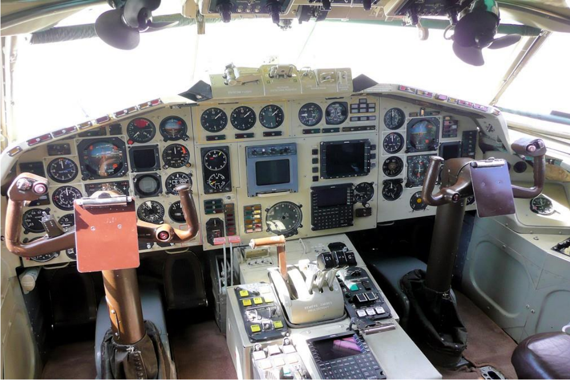
The cockpit of a Polish Tupolev 154M. The approach plates, which normally include the EU OPS 1.405 limits, are attached to the control columns
